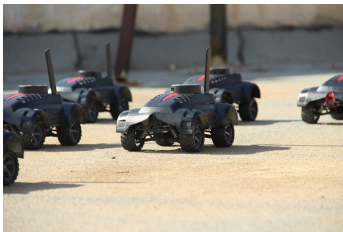
Figure 2: Hamster AUGV; one of the 5 identical robots used in this study.
