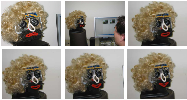
Figure 8: This figure shows continuous changes of the facial expression. Initially, the robot is in a mood corresponding to a blending of sadness and fear since it is alone (top left image). Then, the robot suddenly detects a person and changes its facial expression towards surprise (center image in the first row). Afterwards, the robot gets happy because the person starts to interact with it (following images).
